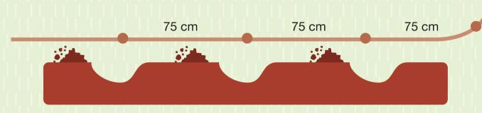
**Plan for measuring and laying out the Basins** = 1 Basin
